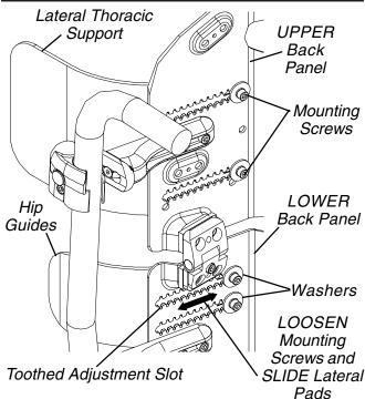
FIGURE 5 - ADJUSTING THE LATERAL SUPPORTS
